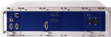
Fig. 2 VC 6000 Monitoring system hardware modules
