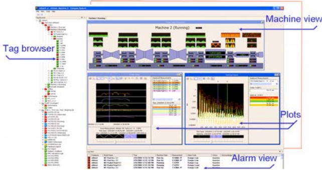
Machine Overview with online safety monitoring software Compass 6000
